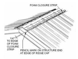
Inside closure strips are to be installed on the underside of the metal roof panels at the eave line and or facia board to prevent insects, vermin and wind driven rain from entering under the metal roof.
